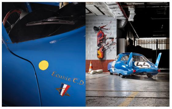
The most noticeable feature of the cars, however, was undoubtedly the twin fin arrangement at the rear that further helped the Panhard to slice through the wind. But without seeing an LM64 in real life, it's difficult to appreciate just how small they they were – a fact that demanded a suitably diminutive engine of just 848cc.
